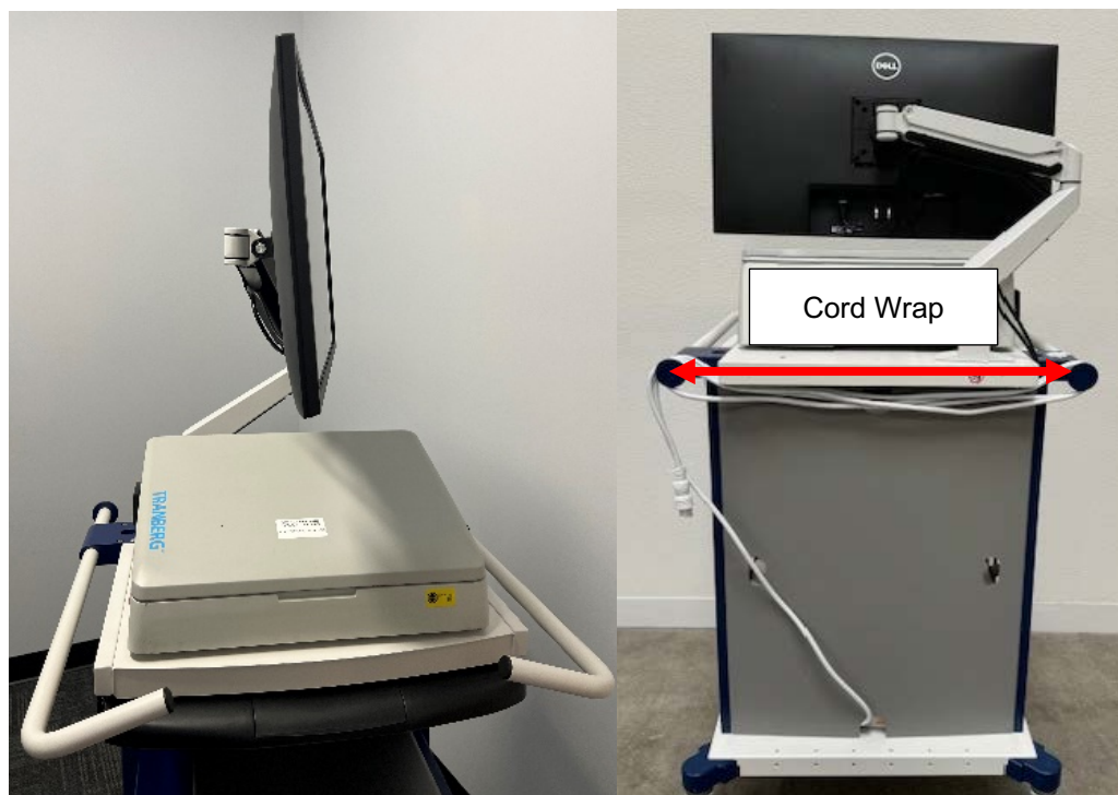
Figure 2. Left: Monitor position during transportation. Right: Power cable managed across Cart cord wrap posts.
